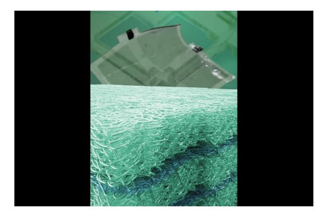
An artificial muscle built from a sandwich of soft, stretchable elastomers and carbon nanotubes electrodes. This type of actuator could be used in everything from wearable devices to soft grippers, laparoscopic surgical tools, entirely soft robots or artificial muscles in more complex robotics. Credit: Peter Allen/Harvard SEAS
