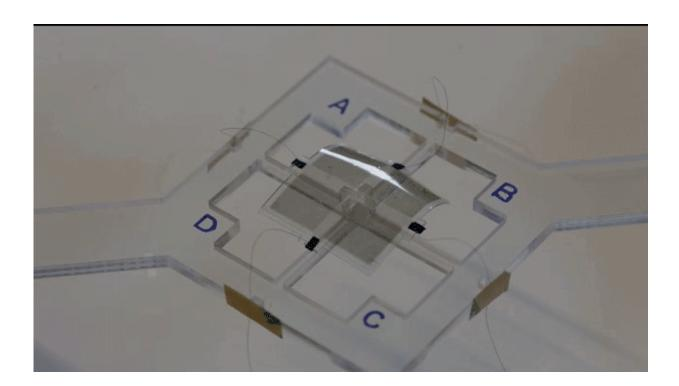
This soft muscle can move with low amounts of electricity. This type of actuator could be used in everything from wearable devices to soft grippers, laparoscopic surgical tools, entirely soft robots or artificial muscles in more complex robotics. Credit: Mishu Duduta/Harvard SEAS
