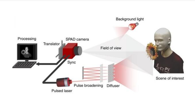
Single-photon camera imaging set-up. Credit: Shin et al.
