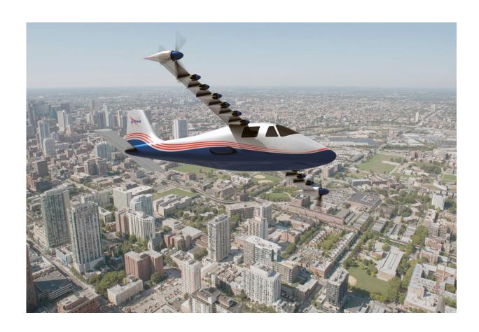
This artist's concept of NASA's X-57 Maxwell aircraft shows the plane's specially designed wing and 14 electric motors. NASA Aeronautics researchers will use the Maxwell to demonstrate that electric propulsion can make planes quieter, more efficient and more environmentally friendly. Credit: NASA Langley/Advanced Concepts Lab, AMA, Inc.
