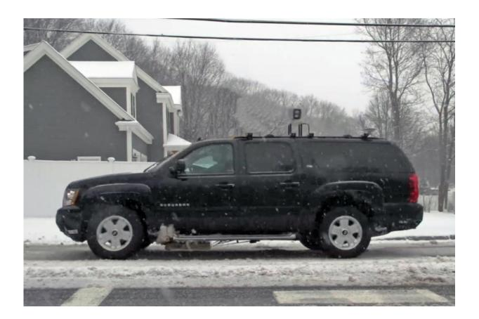
A localizing ground-penetrating radar system mounted beneath this SUV demonstrated centimeter-level localization on snow-covered roads during daytime and nighttime snowstorms. Credit: Massachusetts Institute of Technology
