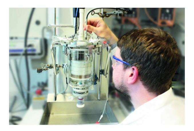
In the future a new sensor will make it possible to analyze the manufacturing process of wall paints and varnishes directly and in real time in the reaction container. Credit: Fraunhofer IAP
