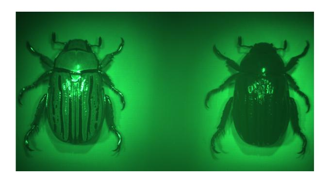
Imaging with the multispectral chiral lens forms two images of the beetle, *Chrysina gloriosa*, on the color camera. The left image was formed by focusing left-circularly polarized light reflected from the beetle and the right image was formed from right-circularly polarized light. The left-handed chirality of the beetle's shell can clearly be seen. Credit:Capasso Lab/Harvard SEAS
