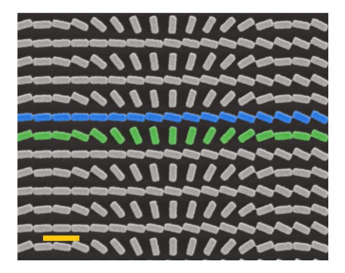
The lens consists of two arrays of titanium oxide nanofins on one glass substrate, as seen below, which forms two images of opposite chirality. Two arrays of titanium oxide nanofins, scale bar 600 nm Credit: Capasso Lab/Harvard SEAS
