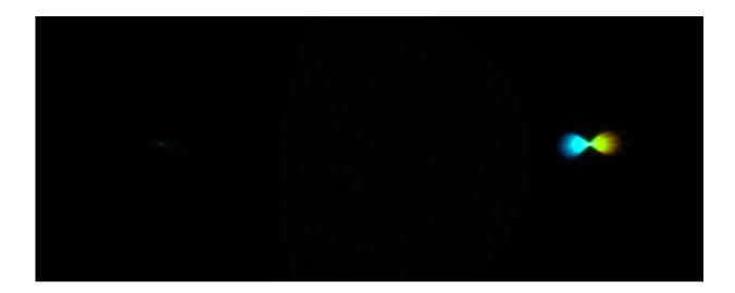
he multispectral chiral lens sorts light based on its chirality and forms two images
