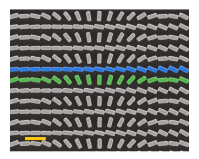
The lens consists of two arrays of titanium oxide nanofins on one glass substrate, as seen below, which forms two images of opposite chirality. Two arrays of titanium oxide nanofins, scale bar 600 nm Credit: Capasso Lab/Harvard SEAS
