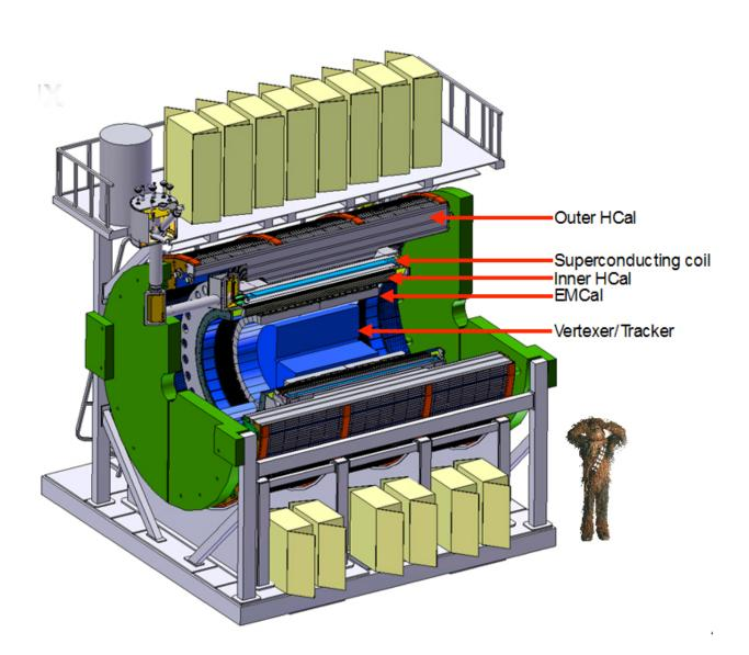
A schematic of the proposed sPHENIX detector, showing several key
