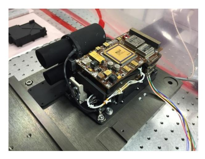
UVIS Flight Model instrument under test. Credit: OU/ESA
