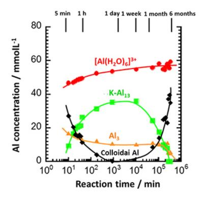
The hydrolysis reaction of aluminum ions. Measurements can be taken a few minutes after the solution is prepared. The measurement process is non-destructive, meaning that the same solution can be monitored over a long period. Credit: Kobe University
