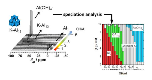
Analysis using 27Al qNMR (quantitative NMR) spectroscopy. Each spectrum can be measured in just three minutes. Credit: Kobe University
