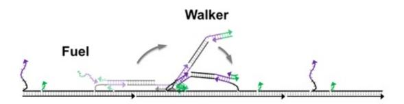
The DNA nanomotor walks using a mechanism called product control, which controls the order in which the products in a chemical reaction are released. This ensures that the nanomotor's back leg always leaves the ground before its front leg. Credit: Liu et al. ©2016 American Chemical Society
