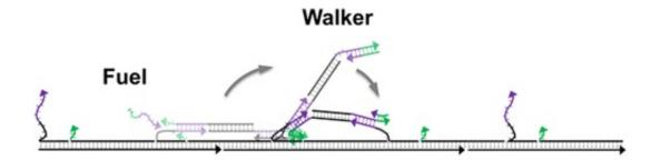
The DNA nanomotor walks using a mechanism called product control, which controls the order in which the products in a chemical reaction are released. This ensures that the nanomotor's back leg always leaves the ground before its front leg. Credit: Liu et al. ©2016 American Chemical Society
