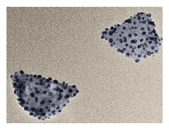
This electron microscope image shows two hybrid nanoparticles, each consisting of a nanodiamond (roughly 50 nanometers wide) covered in smaller silver nanoparticles that enhance the diamond's optical properties. Credit: Min Ouyang
