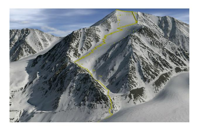
Mt Isto, the tallest peak in the US Arctic, shown as a 3-D visualization of fodar data. Yellow dots indicate position of some of the ground control GPS data collected during the climbing expedition. Closely spaced points are on the climb up, widely spaced points are on the ski down. Credit: Nolan & DesLauriers, The Cryosphere, 2016/Fairbanks Fodar
