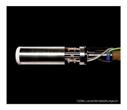
Details of the innovative superconducting coil, conceived and manufactured by researchers from UNIGE and Bruker BioSpin. Credit: L. Windels – UNIGE
