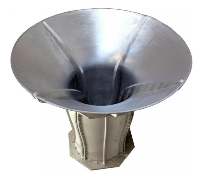
Feed horn for SKA Band 1 in the electronics lab at Onsala Space Observatory. Credit: Onsala Space Observatory/Ronnie Wingdén
