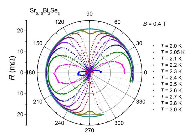
Electrical resistance R, measured for different temperatures. The applied magnetic field rotates in the plane of the layered superconductor. The plot shows that the rotational symmetry is broken. Credit: Fundamental Research on Matter (FOM)
