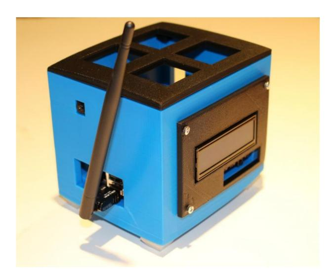
Pi-Sat is a small satellite based on the Raspberry Pi computer. It is low-cost and easy to use, making it ideal for classroom-built satellites. Credit: NASA/Alan Cudmore
