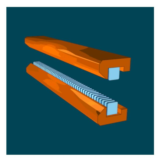
Electrons wiggle between two rows of magnets in a traditional undulator, creating X-rays. These X-rays, or light waves, are linearly polarized. Credit: US Department of Energy
