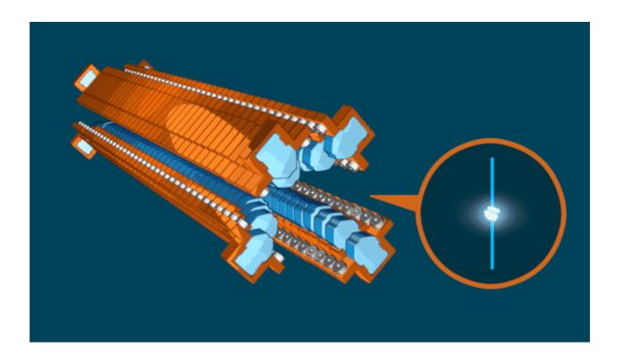
The side-to-side motion of electrons in a beam can be circular, elliptical, or linear, depending on the position of the Delta undulator's magnet rows. These different motions then create circular, elliptical, or linear polarization in the light pulse. Credit: SLAC National Accelerator Laboratory
