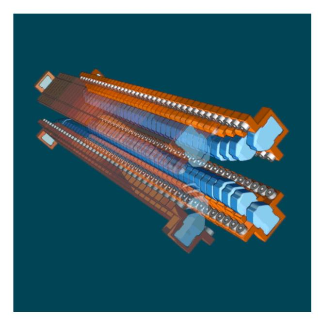
With four moving rows of magnets, the Delta undulator can create circularly polarized, or spiraling, light. Credit: US Department of Energy
