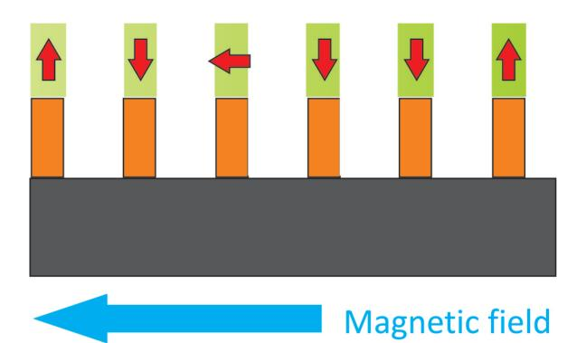
Moderate heating up to 80° Celsius does tilt the magnetic moment associated to a single bit into the plane. Upon cooling to room temperature, the magnetic moment stays in plane, until it is overwritten by a magnetic writing head. Credit: HZB
