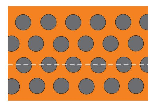
The nanostructured membrane has a honeycomb pattern with nanoholes of 68 nm in diameter. The nanoholes pin down the magnetic domains. Credit: HZB
