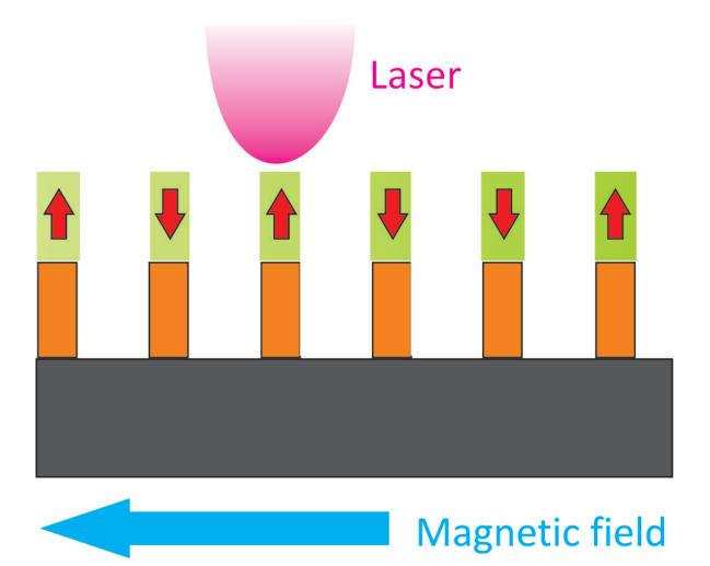
A thin film of Dysprosium-Cobalt (green) has been sputtered on top of the membrane, resulting in an array of antidots. The magnetic moments of DyCo5 are perpendicular to the plane and stable against external magnetic fields. A laser pulse can be used to locally increase the temperature of individual bits. Credit: HZB
