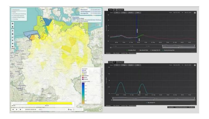
The new demonstration platform "EnergyForecaster" depicts forecasts for the feed of renewable energies in general (left) and for photovoltaics and wind energy in particular (right). Over all, more than 20 different warnings and forecasts can be displayed. Credit: Fraunhofer IWES
