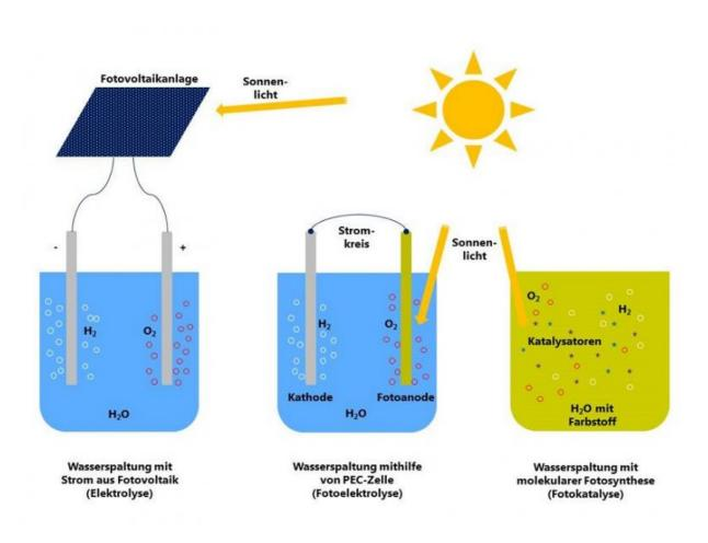
The researchers make a distinction between three different basic approaches to artificial photosynthesis: Photocatalysis is the closest to natural photosynthesis. However, due to its efficiency advantages, photoelectrolysis in PEC cells is currently the main method used. Credit: Empa
