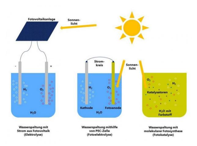
The researchers make a distinction between three different basic approaches to artificial photosynthesis: Photocatalysis is the closest to natural photosynthesis. However, due to its efficiency advantages, photoelectrolysis in PEC cells is currently the main method used. Credit: Empa
