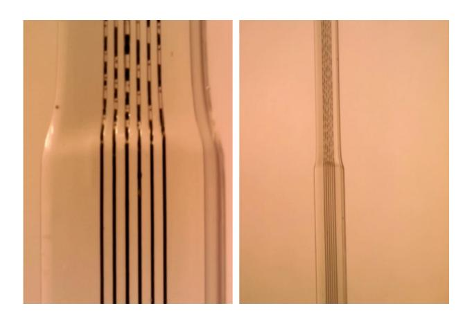
These micrographs show the fibers embedded in polymer and demonstrate how the fibers break apart into segments when they are stretched out in the colddrawing process. Credit: Massachusetts Institute of Technology
