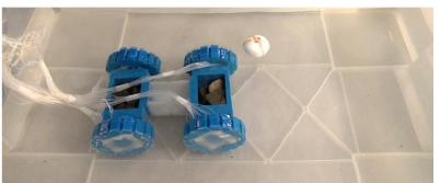
Rutgers University engineers created unique elastomeric rotary actuators based on pneumatically driven peristaltic motion. Using silicone-based wheels, these motors enable a new class of soft locomotion -- not found in nature -- that can withstand impact, traverse irregular terrain and operate in water. For soft robotics, this innovation represents progress toward providing torque without bending actuators. Credit: Xiangyu Gong
