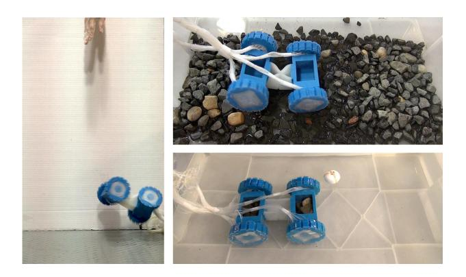
Rutgers University engineers created unique elastomeric rotary actuators based on pneumatically driven peristaltic motion. Using silicone-based wheels, these motors enable a new class of soft locomotion -- not found in nature -- that can withstand impact, traverse irregular terrain and operate in water. For soft robotics, this innovation represents progress toward providing torque without bending actuators. Credit: Xiangyu Gong
