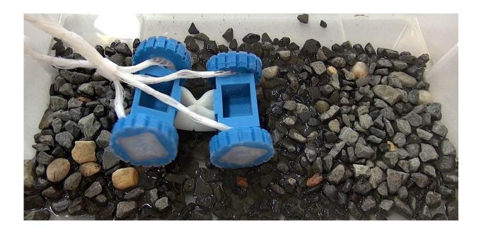
A soft, four-wheeled robotic vehicle powered by a unique soft engine developed
