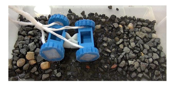
A soft, four-wheeled robotic vehicle powered by a unique soft engine developed
