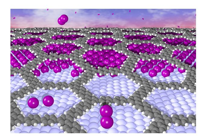
The illustration shows how iodine (purple) is embedded between the organic layer and the metal, thus reducing adhesion. Credit: IFM, University of Linköping
