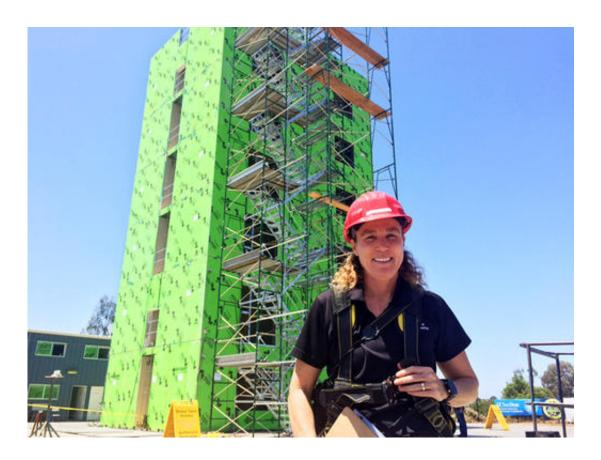
University of California, San Diego structural engineering professor Tara Hutchinson stands in front of a six-story building that is undergoing a series of earthquake tests on a giant shake table, to see how the steel frame structure would fare in a major temblor, in San Diego Wednesday, June 15, 2016. (AP Photo/Julie Watson)
