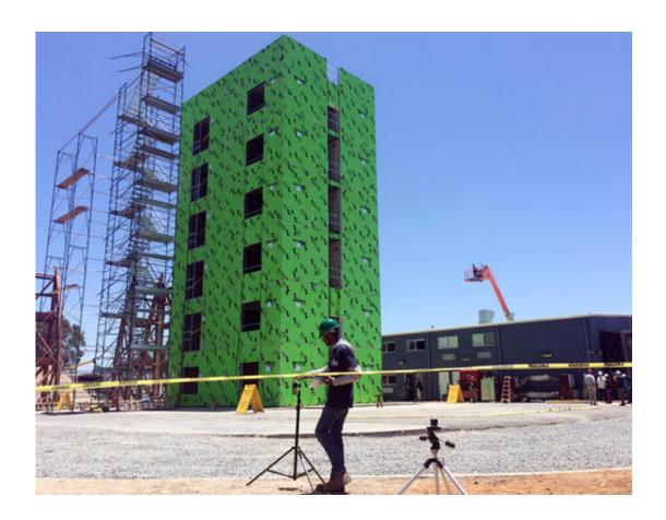
A researcher from the University of California, San Diego checks monitoring equipment in front of a six-story building that is undergoing a series of earthquake tests on a giant shake table, to see how the steel frame structure would fare in a major temblor, in San Diego Wednesday, June 15, 2016. (AP Photo/Julie Watson)
