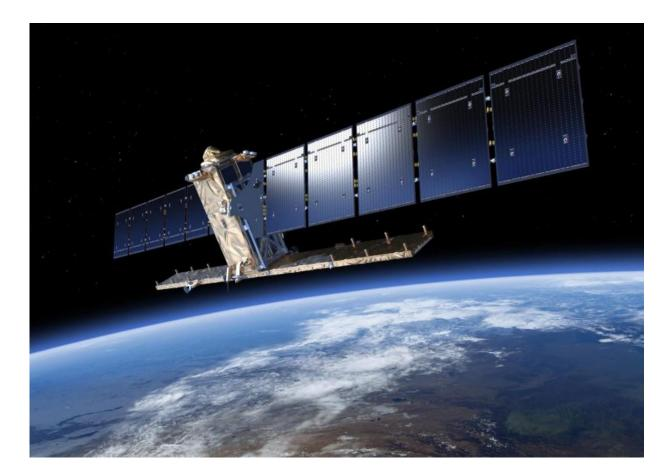
Sentinel-1, the first in the family of Copernicus satellites, is used to monitor many aspects of our environment, from detecting and tracking oil spills and mapping sea ice to monitoring movement in land surfaces and mapping changes in the way land is used. It also plays a crucial role in providing timely information to help respond to natural disasters and assist humanitarian relief efforts. Credit: ESA/ATG medialab
