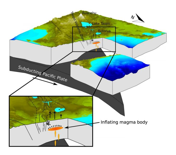
A drawing looking south along the Taupo Volcanic Zone showing the subduction of the Pacific Plate under the North Island of New Zealand. Uplift of the surface measured by satellite radar and GPS suggests the presence of a magmatic body
