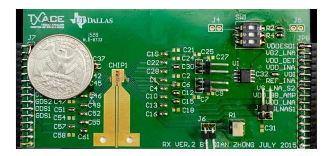
Researchers determined that using integrated circuits, including one shown right of the US quarter and below the label 'CHIP1' in an electronic nose will make the device more affordable. Credit: UT Dallas
