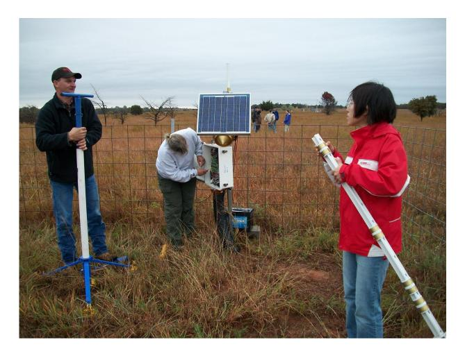
Brice Ruthardt (USDA-ARS) prepares to install a capacitance probe access tube at Site B, while graduate student Geano Dong (Oklahoma State) checks the sensors. Lynn McKee (USDA-ARS) checks the datalogger which will house the data collected. Credit: M. H. Cosh.
