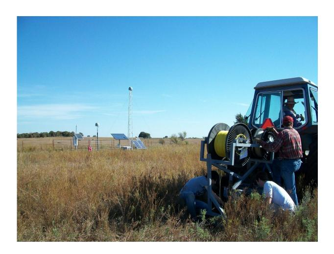
The Distributed Temperature Sensing system is being installed via a plowshear device on the back of a tractor. Graduate students are checking the insertion into the soil trench behind the tractor. Credit: M. H. Cosh.
