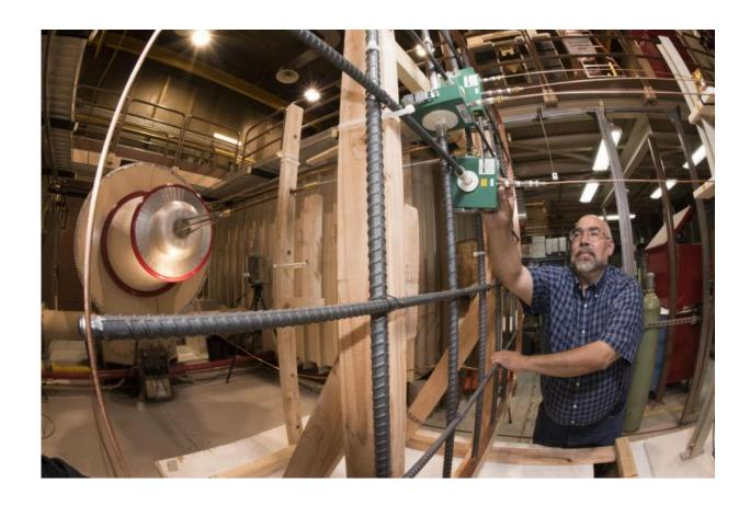
Sandia National Laboratories researcher Leonard Martinez makes an adjustment at the Lightning Simulator lab in a test that's part of a series to further researchers' knowledge of lightning protection systems by looking at how lightning currents flow through rebar lattice structures. Sandia's specialized lightning lab evaluates how everything from sensitive nuclear weapons components to entire buildings will hold up against the worst that nature can offer. Credit: Randy Montoya
