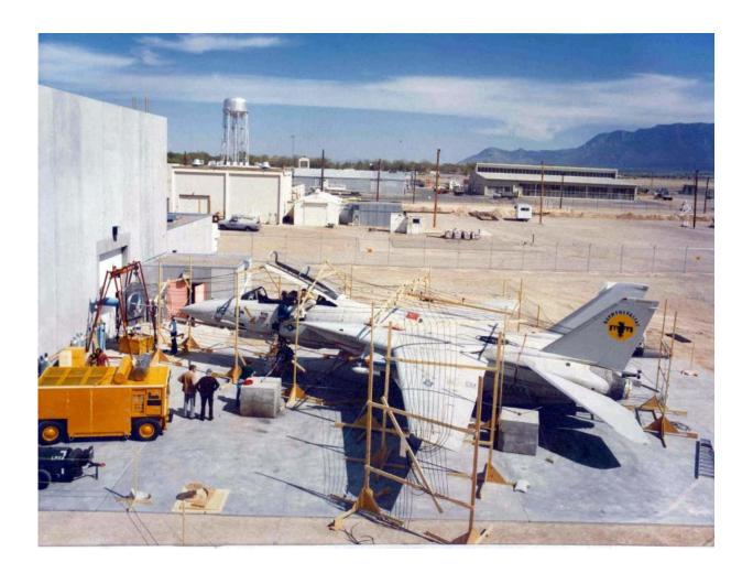
In 1982, Sandia National Laboratories' Lightning Simulator performed a test for the Naval Air Systems Command, which wanted to know how a lightning strike would affect sensitive computer electronics on its aircraft. An F14 was subjected to a charge that entered through the nose and exited via the wing tip. Credit: Sandia National Laboratories
