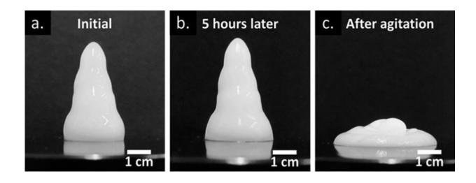
A metal oxide nanoparticle gel (a) resisted flow and behaved as a "pseudosolid" under gravitational forces for five hours (b), but collapsed (c) when agitated with a force greater than the yield stress of the gel, which is the force necessary to make the gel flow. This breakdown of the structure is called "shear-thinning." Credit: Weston et al., Langmuir/American Chemical Society
