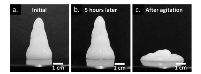
A metal oxide nanoparticle gel (a) resisted flow and behaved as a "pseudosolid" under gravitational forces for five hours (b), but collapsed (c) when agitated with a force greater than the yield stress of the gel, which is the force necessary to make the gel flow. This breakdown of the structure is called "shear-thinning." Credit: Weston et al., Langmuir/American Chemical Society
