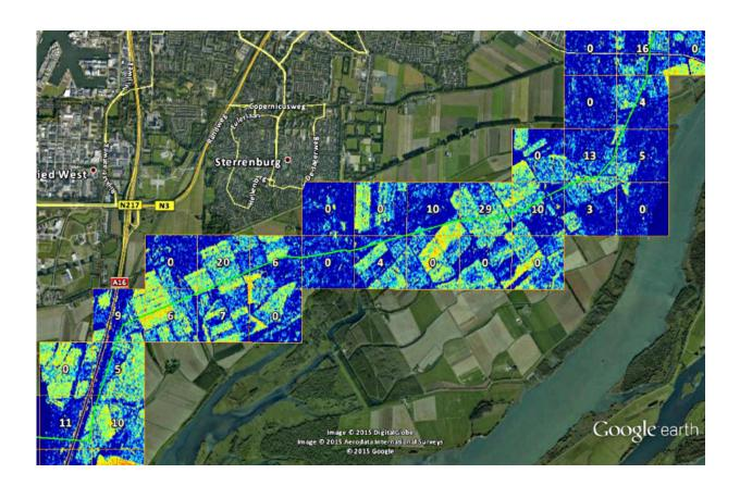
PIMSyS was developed by Dutch company Orbital Eye within ESA's Integrated Applications Promotions programme. The service uses Earth observation data and satcoms to monitor gas and oil pipelines and increase safety. Radar satellite data superimposed on Google Maps imagery indicates land use adjacent to a gas pipeline in the Netherlands. Credit: ESA
