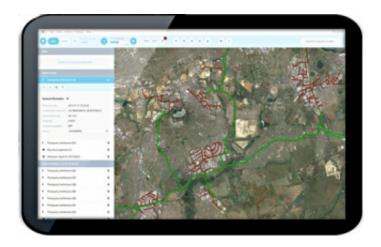
PIMSyS was developed by Dutch company Orbital Eye within ESA's Integrated Applications Promotions programme. The service uses Earth observation data and satcoms to monitor gas and oil pipelines and increase safety. Credit: ESA
