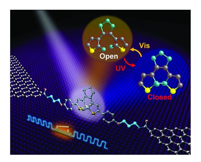
Schematic of a graphene-diarylethene-graphene junction that highlights the expansion of the molecular bridge by methylene groups. Credit: (c) *Science* (2016). DOI: 10.1126/science.aaf6298
