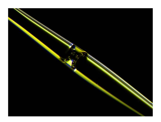
Photograph of a fluid meniscus inside an opto-mechano-fluidic resonator (OMFR) made of high purity silica glass. Particles flowing through the internal microchannel can be detected optically at extremely high speed. Credit: University of Illinois
