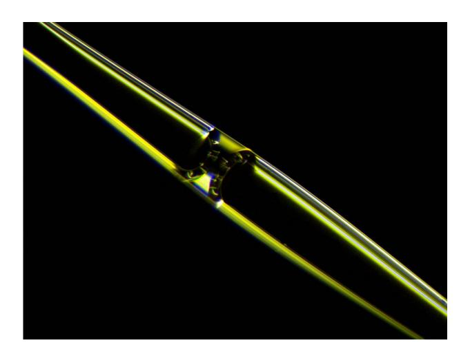
Photograph of a fluid meniscus inside an opto-mechano-fluidic resonator (OMFR) made of high purity silica glass. Particles flowing through the internal microchannel can be detected optically at extremely high speed. Credit: University of Illinois
