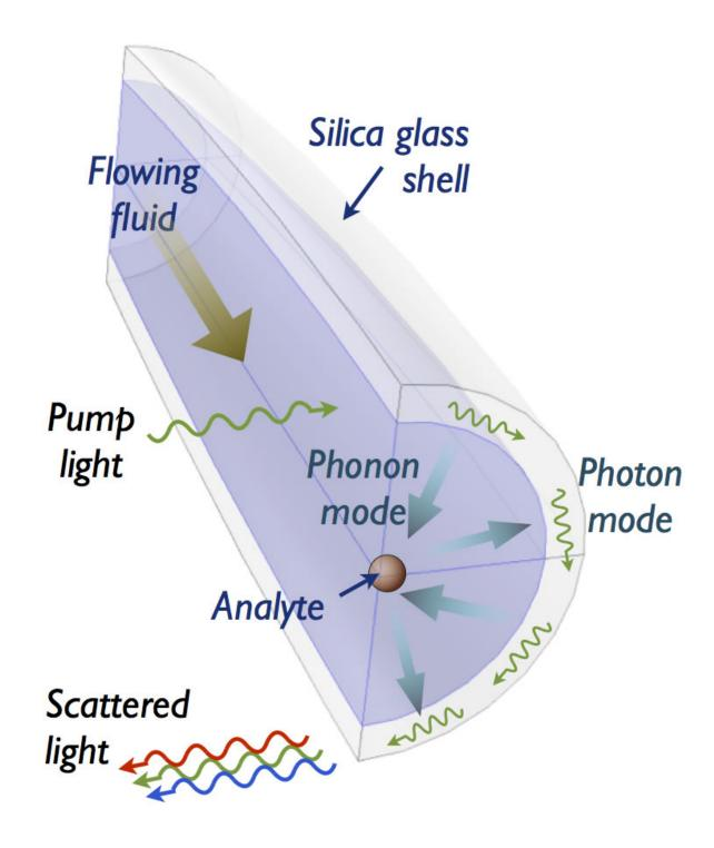
OMFRs employ phonons (quasiparticles of sound and vibration) to engage the conversation between the flowing analyte particles and circulating photons (particles of light) in the silica glass shell. In doing so, they make light sensitive
