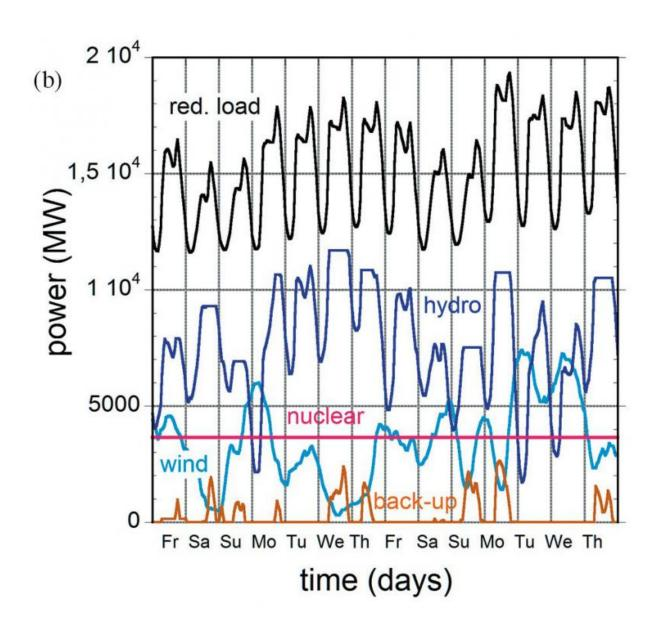
The figure shows the reduced load along with the original nuclear power, the
