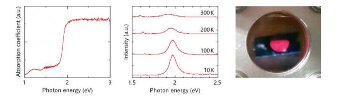
Figure 2. Optical properties of CaZn2N2. Left: Photoabsorption spectrum. Middle: Photoluminescence spectra at temperatures of 10, 100, 200, and 300 K. Right: Photograph of red photoluminescence at 10 K. Credit: Tokyo Institute of Technology
