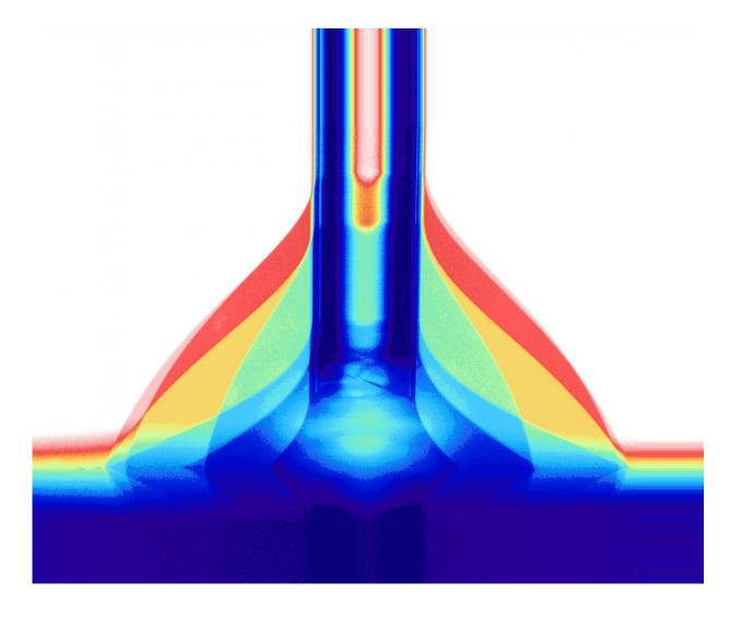
Electrochemistry in a drop: superposition of seven dynamic contact angle measurements of a drop of water on a surface; diameter of vertical tube capillary 0.85 mm. Credit: University of Zurich
