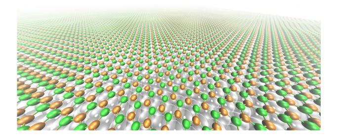
Flattened boron nitride nanomesh with intercalated hydrogen: hydrogen (white), nitrogen (green), boron (orange), rhodium (grey); distance boron-nitrogen: 0.14 nm. Credit: Marcella Iannuzzi, UZH & Ari Seitsonen, ENS Paris
