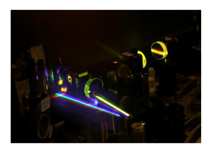
Optical elements of the experimental setup allowing to obtain visible-spectrum laser pulses as short as 10 femtoseconds. Credit: Dr. R. Borrego-Varillas and Prof. G. Cerullo, University Politecnico Milan (Italy), Author provided
