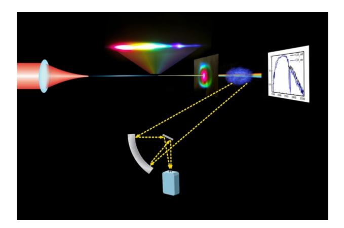
This diagram depicts the way a mid-infrared laser (red cylinder, left) can send a beam through the atmosphere that generates filaments of ionized air molecules (multicolored beam, center, shown with magnified view). These filaments, which can be kilometers long, help to keep the beam concentrated enough to generate mid-infrared light in air (blue cloud, right) that can reveal detailed chemical composition through spectral analysis (chart at right) of the light picked up by a
