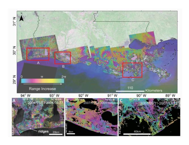
The red frames show the location of enlarged interferograms presented in Figures A, B and C. A) Radarsat-1 interferogram of the western Chenier Plain spanning 24-day period (2004/01/03-2004/01/27). In the central part of the interferogram fringe patterns show changes in inland water bodies. The left side of the interferogram shows fringe patterns due to the morphology of the Chenier reflecting water level changes in the mudflats in between the ridges of the
