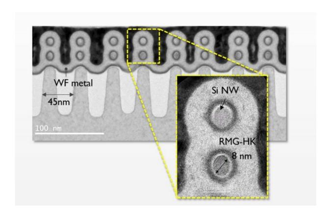
TEM images of an NMOS GAASiNWFET(LG=70nm):(a)overview of the SiNW array; (b)detailed view of two stacked SiNWs. Credit: IMEC RSS feed
