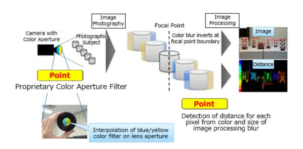
Researchers have developed an imaging technique that can simultaneously acquire a color image and a depth map from a single image taken by a monocular camera. This technique achieves highprecision distance/range detection, comparable to that of a stereo camera, through the combination of a lens device and image processing.
