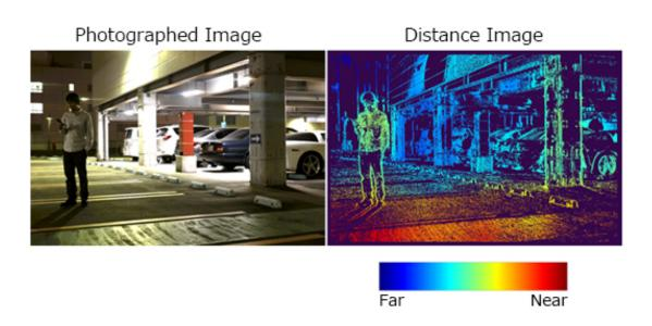
Thus, conventional distance sensors have a variety of advantages and disadvantages. Obtaining a high degree of accuracy in a compact low-cost package is difficult.
