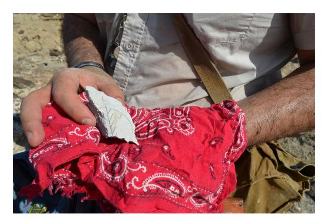
A tuff sample chiseled out for later lab analysis. Lepre has etched an arrow into the sample to indicate which way pointed north before he removed it. Credit: Columbia University
