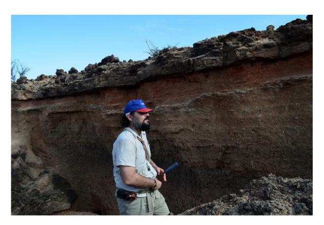
Lepre prepares to sample an outcrop of ancient sediments. He establishes the ages of objects found within or near layers using magnetostratigraphy--the study of how earth's magnetic field periodically reverses itself. Changes in polarity can be identified by the orientation of mineral grains. Credit: Columbia University
