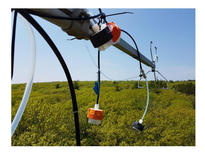
Flux towers are equipped with inlets for "sniffing the air" above the forest, in addition to other instruments such as sonic anemometers for measuring wind. Credit: Richard Wehr
