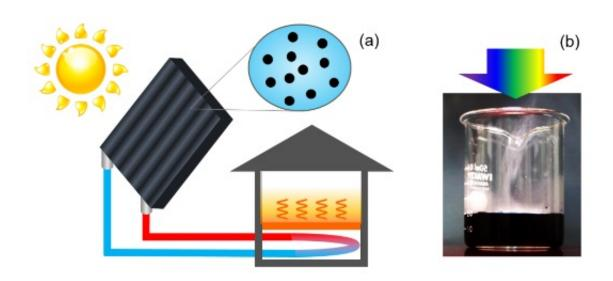
Figure: (a) Diagram showing a solar water heating system using nanoparticles. (b) Application of condensed light from a solar simulator to water with dispersed TiN nanoparticles. Note that rising water vapor can be seen even before the water temperature increases. Credit: NIMS
