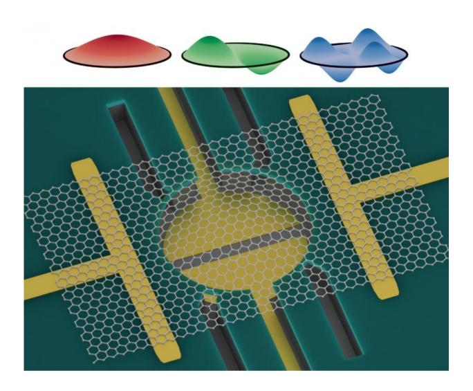
Top: Three vibrational modes excitable in circular drums. In graphene, these modes are coupled to one another and can exchange energy. Bottom: An artist's depiction of a graphene drum. The graphene vibrates above a circular trench on a silicon chip. T-shaped metal electrodes contact the graphene's bottom surface,
