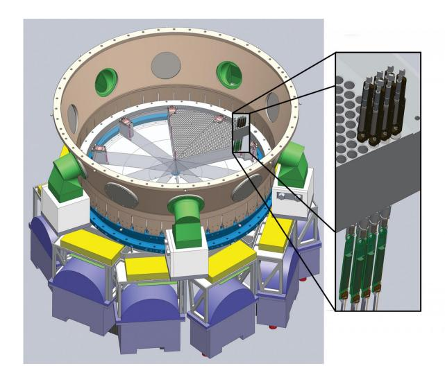
An array of 10 wedge-shaped petals, each loaded with 500 robotic fiber-optic positioners, will be assembled in the Dark Energy Spectroscopic Instrument's focal plate. At right, a view of the robots fitted into holes in one of the petals. Credit: DESI Collaboration
