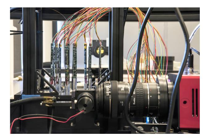
A view of the ProtoDESI setup under assembly at Berkeley Lab, with the underside of the robotic fiber-positioners visible at left. Credit: Paul Mueller/Berkeley Lab
