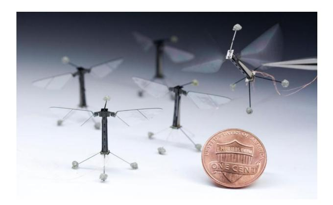
Inspired by the biology of a fly, with submillimeter-scale anatomy and two waferthin wings that flap almost invisibly, 120 times per second, the Robobee takes its first controlled flight. The culmination of a decade's work, RoboBees achieve vertical takeoff, hovering and steering. Credit: Kevin Ma and Pakpong Chirarattananon
