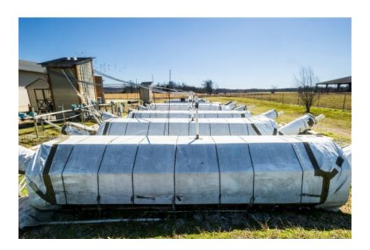
Pilot-scale anaerobic digestion reactors at the USDA Beltsville Agricultural Research Center. The replicate digesters, designed by University of Maryland researcher Stephanie Lansing, will be used in the new study. Credit: Edwin Remsberg/University of Maryland
