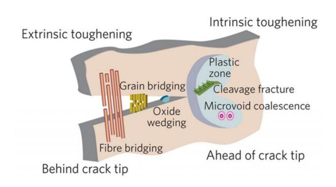
Materials used for their mechanical strength employ a variety of toughening mechanisms. At the nanoscale, intrinsic toughening mechanisms that promote flexibility occur in front of a moving crack. At larger length scales, extrinsic toughening mechanisms, specifically those that help reduce the stress that forces the crack to advance and grow, act mostly behind the crack tip. Credit: US Department of Energy
