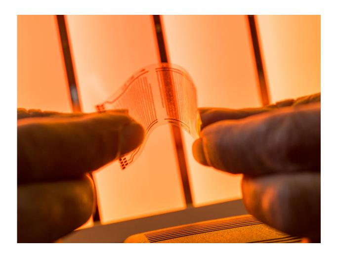
The EXTMOS project will help develop new organic semiconductor materials and additives that can be printed onto flexible film to create devices that are low cost, flexible, wearable and lightweight. Credit: Nic Delves-Broughton, University of Bath
